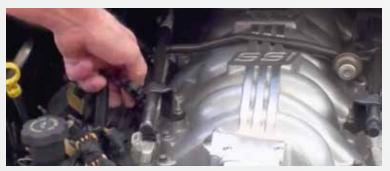
Unplug the electrical connections from the fuel injectors.
