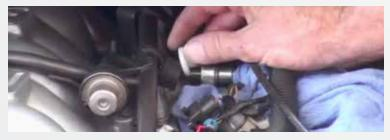
Hold a rag around the shrader valve on the front of the driver side rail, and then bleed off any fuel pressure by depressing the valve with a small pick tool.
