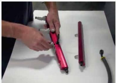
Insert (4) injectors into each rail.
