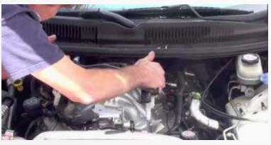
Remove the fuel rails and injectors by simply lifting them straight up.
