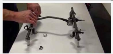
Remove the clips that retain the injectors in the rails.
