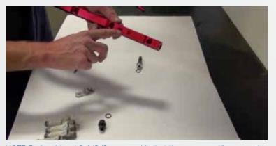
NOTE Each rail has LS-1/2/3 engraved in it at the corresponding mounting tab holes. Attach the mounting tabs at the proper location for your engine designation.
