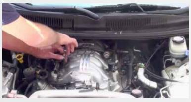
Use a 10mm socket to remove the bolts that attach the fuel rails to the intake manifold, and an 8mm socket to remove the small L shaped bracket that attaches to the fuel rail stud on the passenger side. Corvette models may require that you remove the intake manifold bolts and slide it forward to remove this bracket. STEP 7
